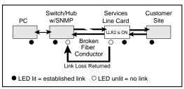
If LLR is disabled and the fiber port's receiver loses link, the port's transmitter behavior will depend on the auto-negotiation setting. If auto-negotiation is enabled, the transmitter will shut down. If auto-negotiation is disabled, the transmitter will continue to stay up. The following table describes the transmitter's response when the port stops detecting link, based on the LLR and auto-negotiation settings.
