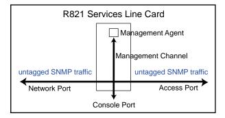
Through software, you can create a secure management channel by assigning it a new management VID<sup>2</sup>. The most secure configuration is to have only one port (typically, the network port) enabled for management. This is the recommended configuration, and it allows you to restrict access to the card's management agent, thus preventing unauthorized modifications and other misuses.
