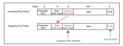
The data remains unchanged. Logical Services Loopback operates at full line rate with frames of any size. Normal data frames continue to be received and transmitted without being dropped while Logical Services Loopback is enabled.
