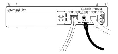
**Note:** Do not remove the dust plug from the console port until you are ready to connect the console cable to the port. When you remove the console cable, please replace the port's dust plug.
