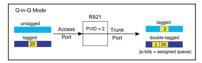
If a received frame contains DSCP and/or p-bit elements, and the respective classification mode(s) is/are enabled, then that information will be used to perform internal queuing, otherwise the access port's default port priority will be used for queuing.
